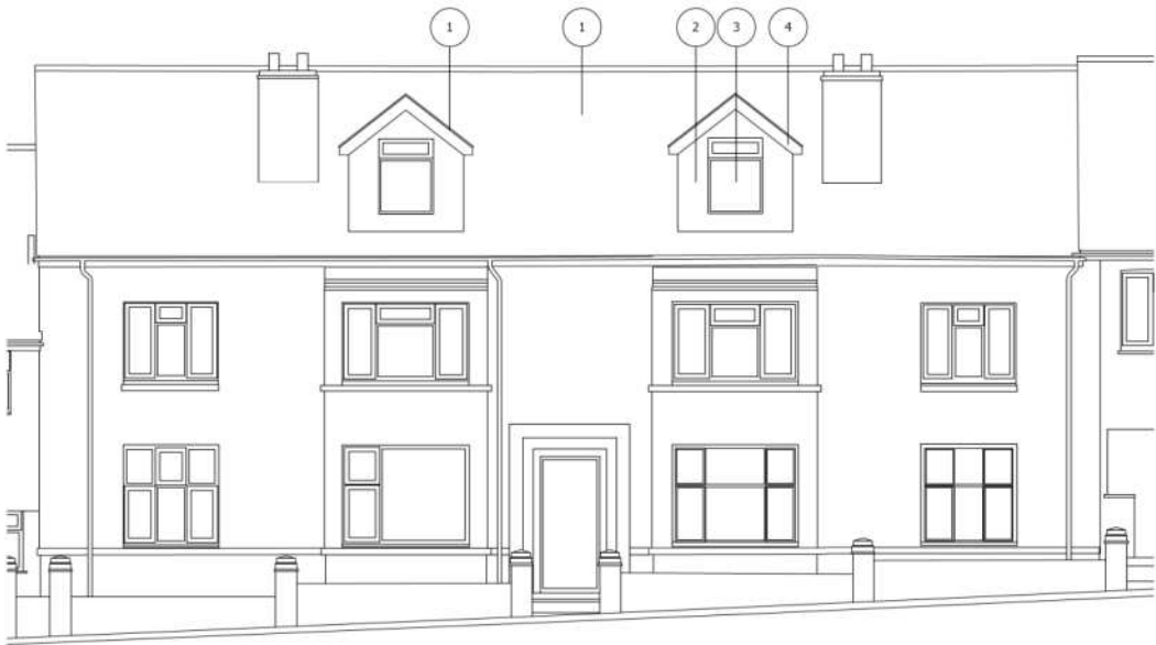
9 Proposed Front Elevation Scale: 1:100
